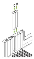
Note: The SupremeRAID™ SR-1010 is dual-slot card and requires you to remove two adjacent slot covers. The SupremeRAID™ SR-1000, SR-CORE-AM, SR-PRO-AM, SR-ULTRA-AD and SR-1001 are single-slot cards and require only a single- slot.
