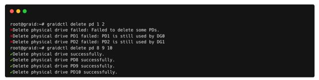
The output shows that a physical drive cannot be deleted when it is part of a drive group.
