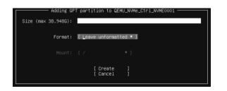
Note: You must use [Leave unformatted]. DO NOT mount the partition. Setting RAID1 and mounting partitions on multiple drives (MD) occurs later in this procedure.
