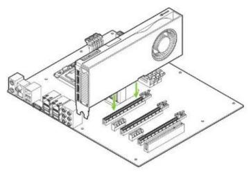
Note: Install the SupremeRAID<sup>™</sup> card into the primary x16 PCI Express slot. The SupremeRAID<sup>™</sup> SR-1010 is dual-slot card and covers the adjacent slot. The SupremeRAID<sup>™</sup> SR-1000 and SupremeRAID<sup>™</sup> SR-1001 are single-slot cards. For more information, see <u>https://manuals.plus/nvidia/rtx-ampere-architecture-based-graphics-card-manual#ixzz7wk7PysLh</u>.
