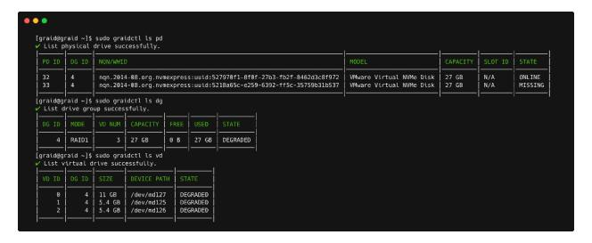
The following example shows a replaced drive. The bootable RAID group rebuilds immediately after replacing the drive.
